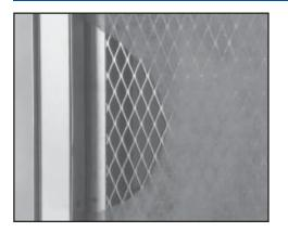
An Expanded Stainless Steel Media Support forces particulates to impregnate the media, layer heavily and accumulate across its surface, until efficiently rolled onto the Used Media take-up roll.
